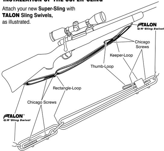
Overall length of your Super-Sling can be increased by repositioning the webbing and Chicago Screws as illustrated in the diagram below.
